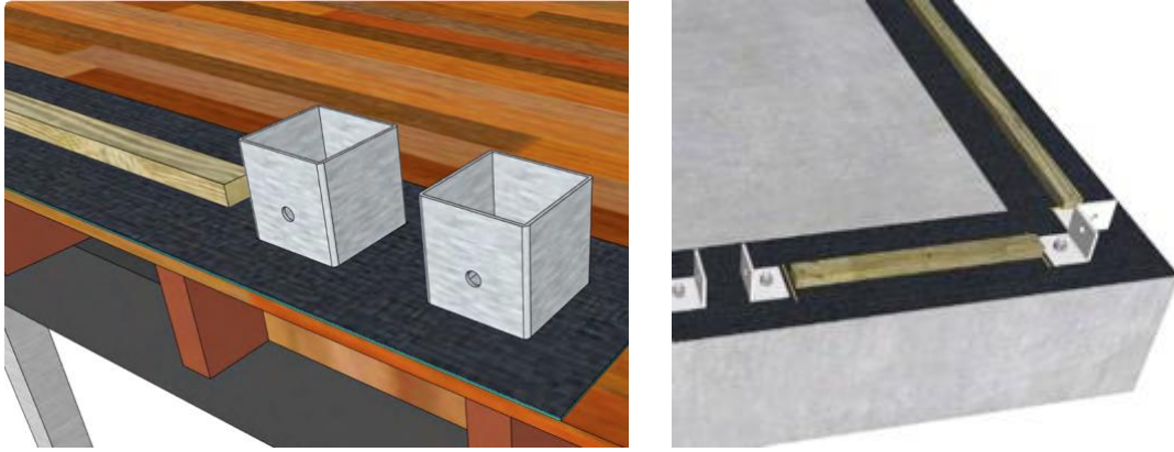
Figure 27 - Steel foot (stanchion) installation
