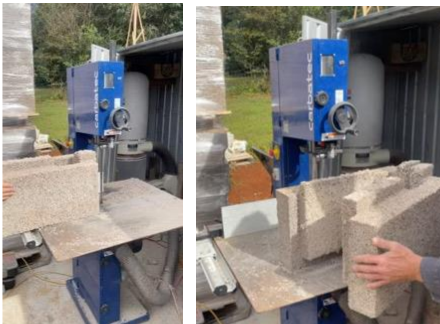
Figure 35 - Cutting a block over long
