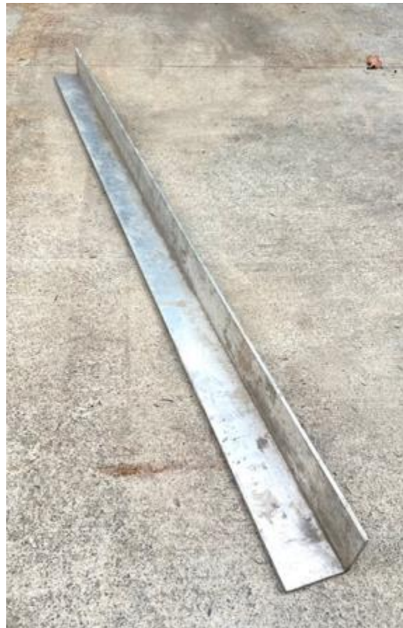
Figure 67 - Aluminum support angle
