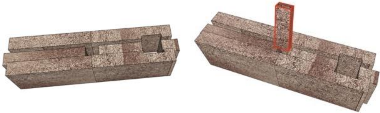
Figure 40 - Filling the void at two grooves
