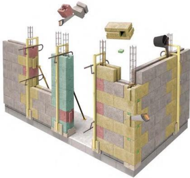
Figure 79 - The steel reinforced system
