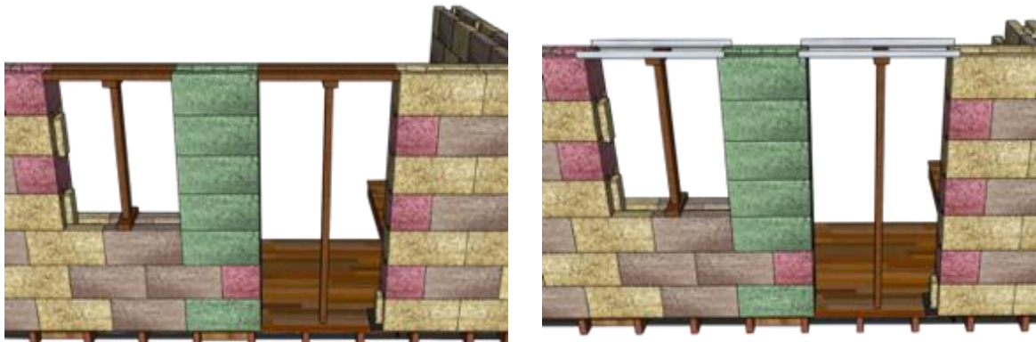
Figure 68 - Installing temporary supports
