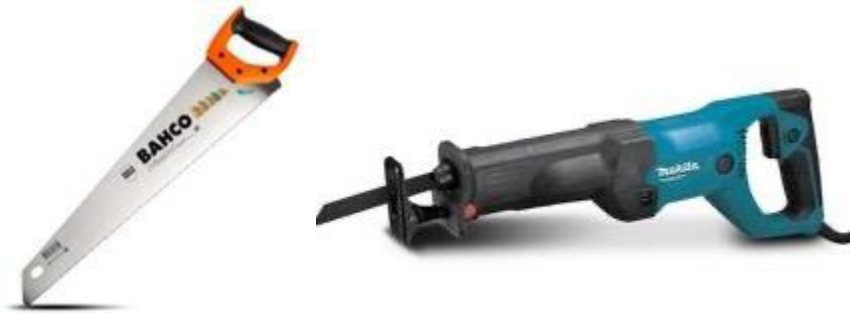
Figure 3.1 - Tools for cutting HempBLOCKs
