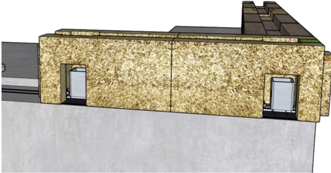
Figure 39 - Cutting out access holes
